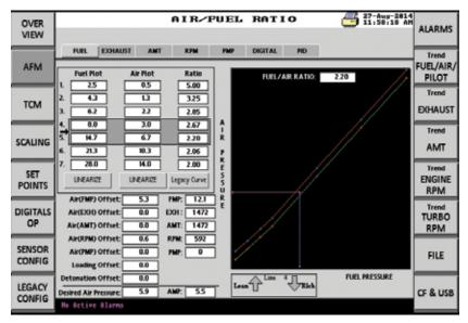
When replacing an EPC-200, enter the existing three point values of the air/ fuel curve by pressing the Legacy Curve button.
