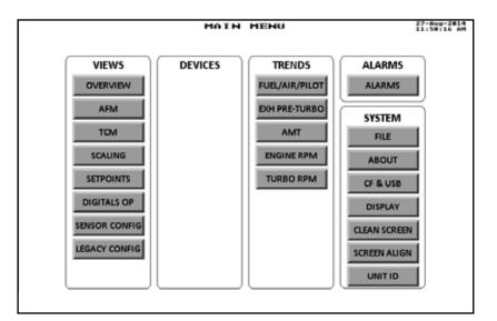
6.3 Press LEGACY CONFIG to view the configuration screen for the legacy EPC-200 inputs.
