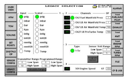
When replacing an existing EPC-200, the end devices require configuration within this screen as described below prior to calibrating any channel.
