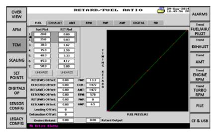
The operating values for the functions above are calculated separately according to user-entered curves, and the Offset is implemented by the EPC-250 Controller.
